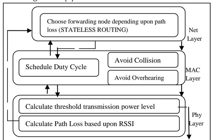
Figure 5.1. Cross layer design of the proposed protocol
