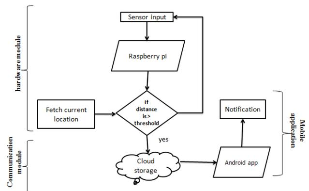
Fig.8: Operational details of pothole detection
