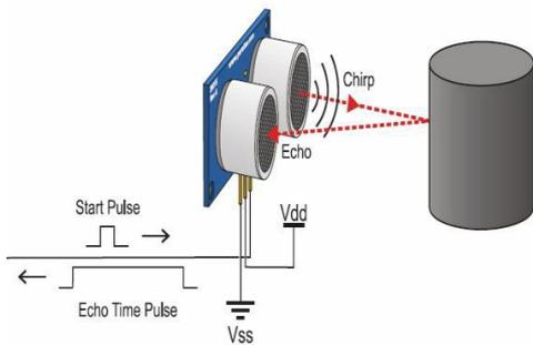
Fig. 3: Ultrasonic sensor (HC-SR04)
