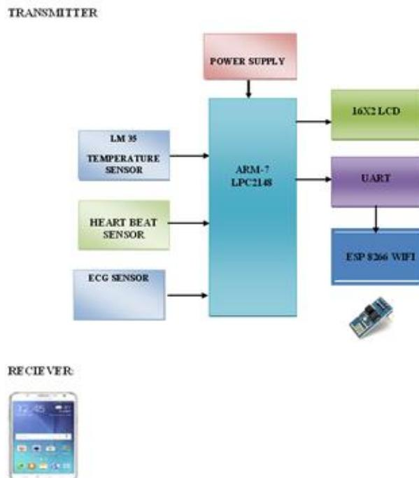
Figure 2. Block Diagram
