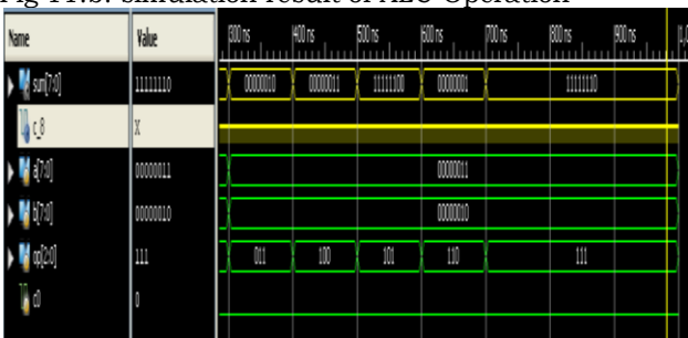
Fig 11.c: simulation result of ALU Operation
