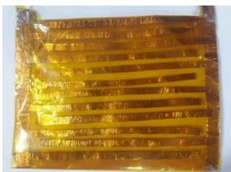
Fig. 2. Prototype of electroadhesive pad using polyimide film.
