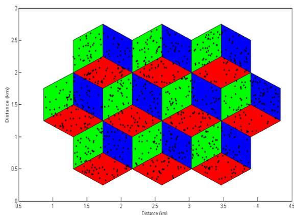
Figure 1: Cellular layout where the users are randomly spread in the entire cell area with nine cells. There is no separation of users as cell center and edge.
