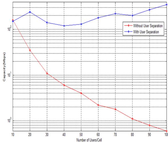
Figure. 3. A plot for the average cell throughput versus number of users considering cell radius as 450m and users ranging from 10-100 users.
