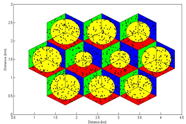
Figure. 2. Cellular layout where the users are randomly spread in the entire cell area with nine cells. There is separation of users as cell centre and edge indicated by a varying circular structure.
