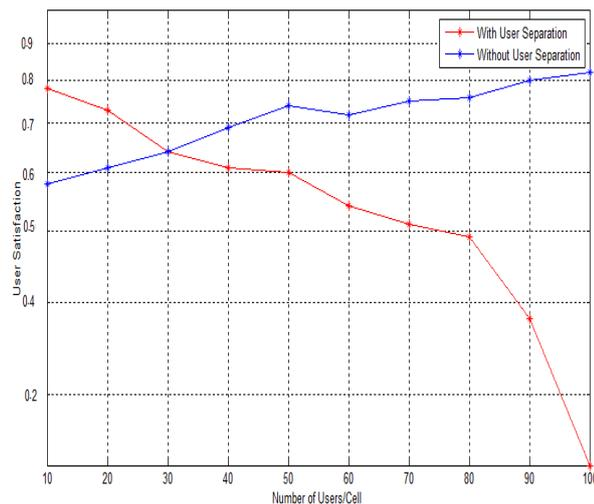
Figure. 4. A plot for average User Satisfaction for respective throughput, number of users considering cell radius as 450m and users ranging from 10-100 users.
