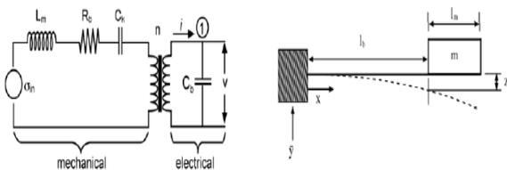
Figure 2. (a) Circuit representation of the piezoelectric generator. (b) A schematic diagram of the generator.
