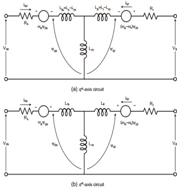
Figure 2: Synchronous frame (de-qe) dynamic model equivalent.
