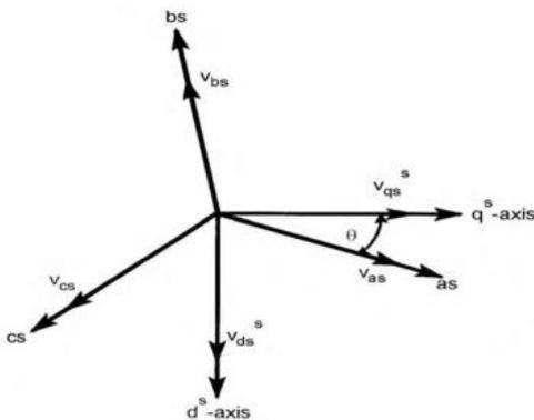
Figure 1: Stationary frame (as-bs-cs to ds-qs) transformation. The 3-phase frame as-bs-cs are converted into 2-phase ds-qs frame.
