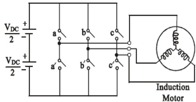
Figure 4: Power circuit connection diagram for the Induction motor.
