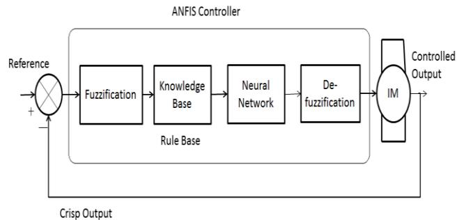
Figure 6: Block diagram of the ANFIS control scheme for the speed control of the IM.
