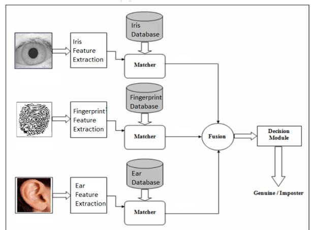
Fig 8: Architecture of proposed multimodal biometric recognition system integrating iris, fingerprint and ear.
