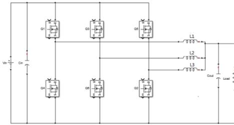
Fig. 3 : Simulation circuit of three-phase synchronous buck converter.
