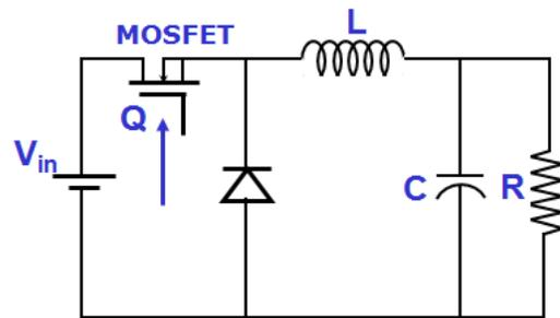
Fig. 1 : Conventional Buck Converter
