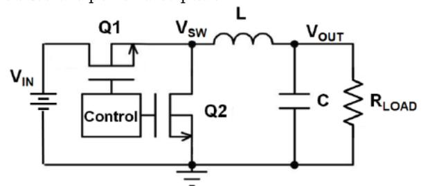
Fig. 2: Synchronous Buck Converter
