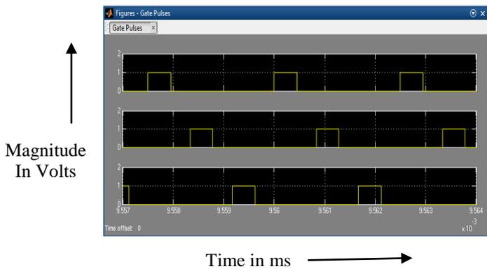
Fig. 3.1 : Gate pulses for three-phase synchronous buck converter.
