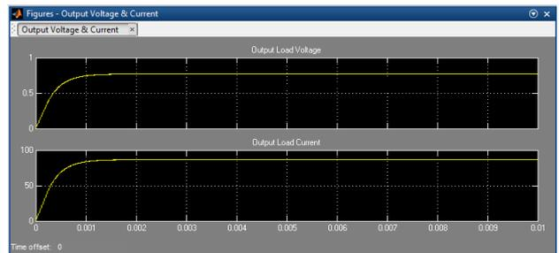
Fig. 3.3: Output voltage and output current of the three-phase synchronous buck converter.
