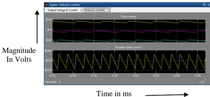
Fig. 3.2: Phase currents and phase current ripples of three-phase synchronous buck converter.
