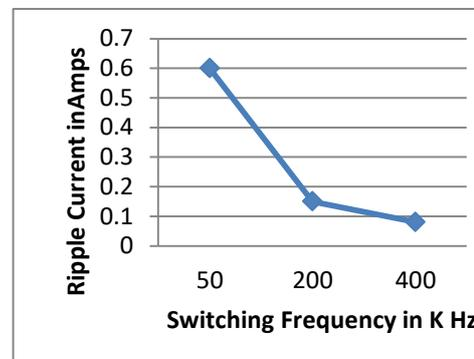
Fig..3.4: Graph of Ripple Current Vs Switching Frequency
