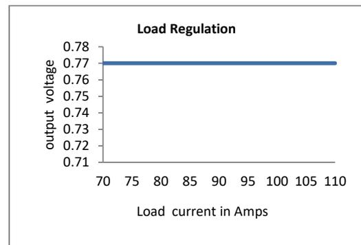
Fig.3.7. Graph of Load Regulation
