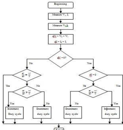
Fig. 3: Flowchart of Incremental Conductance algorithm
