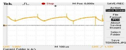
Fig. 10: Inductor current obtained from Buck Converter
