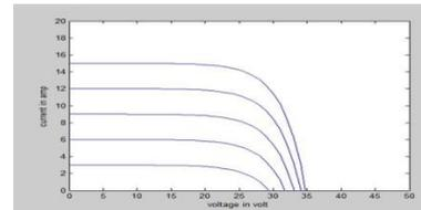
Fig. 5: Solar VI characteristics obtained through programming in MATLAB for various insolation
