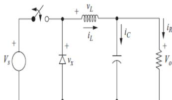
Fig. 4: Schematic of Buck Converter
