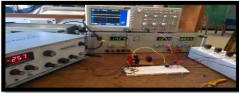
Fig. 8: Hardware Implementation of Buck Converter using MOSFET as a Switch
