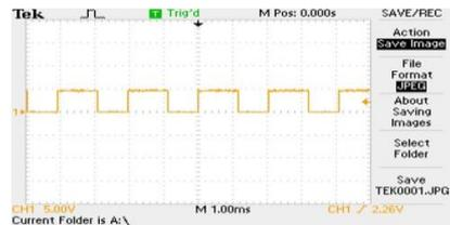
Fig. 11: Switching Pulses from ATMEGA328P which are given to MOSFET
