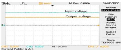
Fig. 9: Results of Hardware Implementation showing input voltage (12 V) and output voltage (6.5V) for a duty cycle of 0.5
