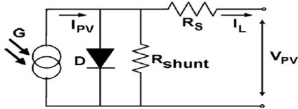
Fig. 1: equivalent model of solar cell
