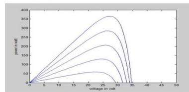
Fig. 6: Solar PV characteristics obtained through programming in MATLAB for various insolation
