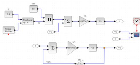
Fig. 7: Mathematical model of Buck Converter in Xcos Tool of Scilab
