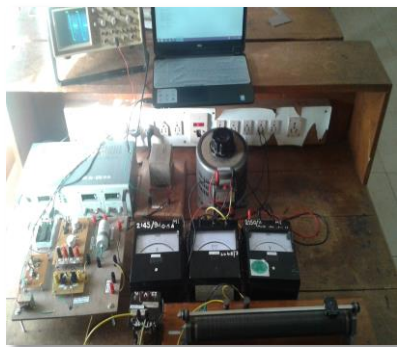
Fig.13. Hardware Testing of the SVC circuit
