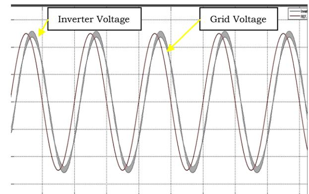
Figure 6(c): Inverter voltage and Reference (Grid)Voltage Waveforms.
