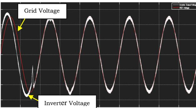
Figure 7(b): Inverter and Grid control voltage waveforms.
