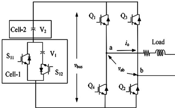
Figure 1. Proposed Single Phase Five Level Inverter
