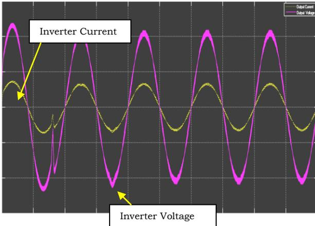
Figure 7(a): Inverter voltage and current waveforms when grid control signal is connected
