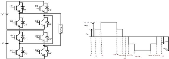
Figure 1. a) 5-level inverter b) 5-level waveform
