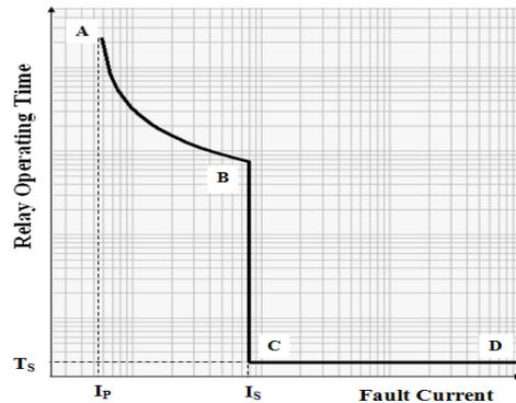
Fig.2. Current Time Characteristics of an Over-Current Relay
