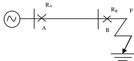
Fig.4.Radial feeder for single phase system
