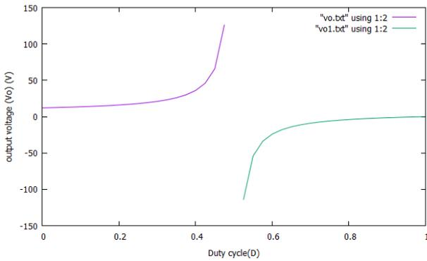
Fig. 5 Voltage gain as a function of d
