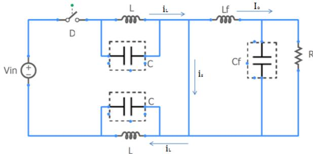
Fig. 3 Equivalent circuit of the Z-source dc-dc converter when S is ON and D is OFF.
