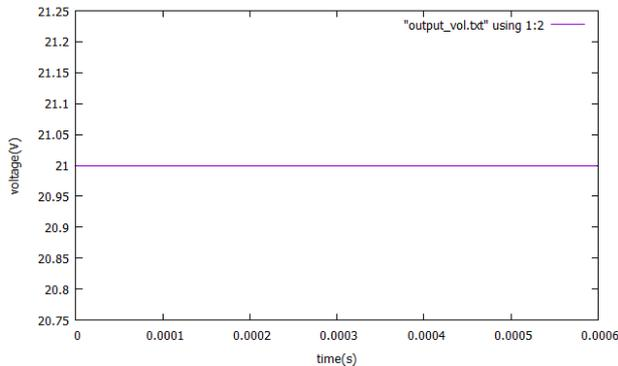
Fig. 11 Z-source DC-DC converter output voltage waveform
