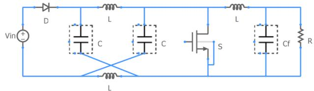
Fig. 2 Z-source DC-DC converter topology
