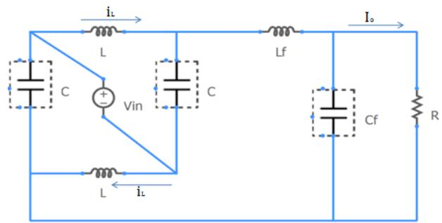
Fig. 4 Equivalent circuit of the Z-source dc-dc converter when S is OFF and D is ON.
