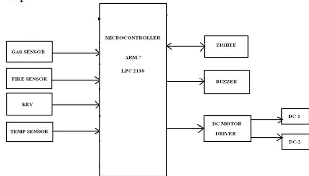
Figure.1 Block diagram of Mine Monitoring System
