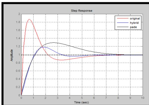
Figure.3 Comparisons of original system with reduced lower order systems by various approximations
